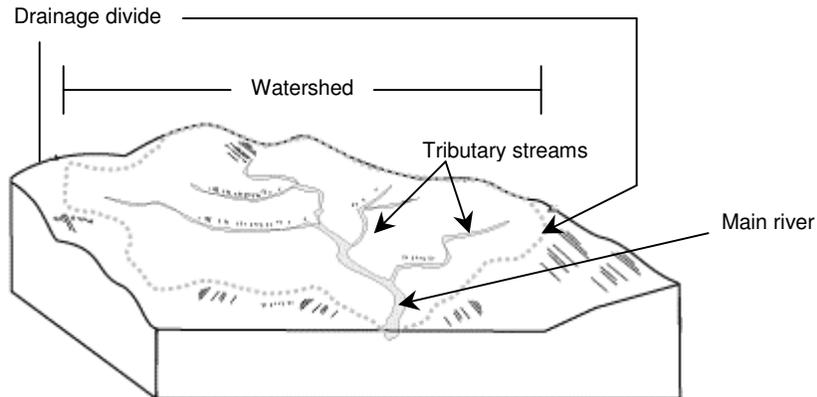
**Figure 3.8-1 Watersheds** A watershed is the land area that drains to a common location (typically a water body and its tributaries). For this reason, watershed boundaries are also called drainage divides. Practices to reduce the temperature of runoff must be installed if a site is located anywhere within the watershed of a thermally sensitive water body. Figure 3.8-2 shows these water bodies and the boundaries of their watersheds.
