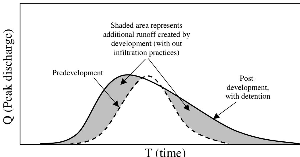
**Figure 3.1-5 Hydrograph with stormwater detention practices installed**
