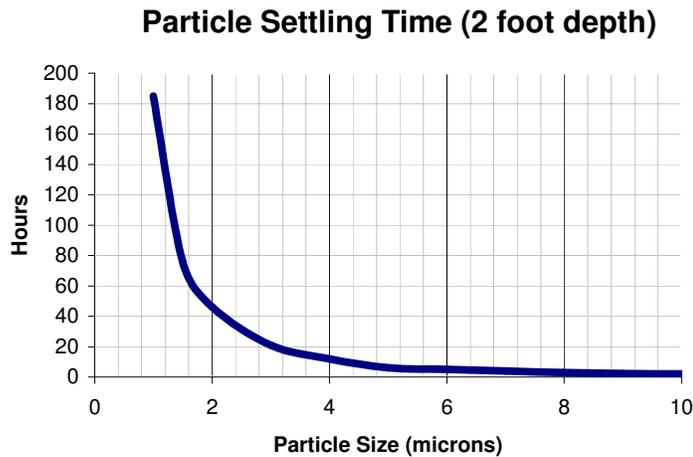
Figure 2.3-2 Particle Settling Time
