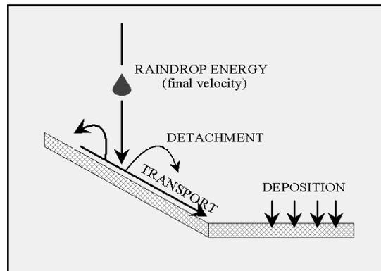
**Figure 2.1-1 Conceptual Model of Erosion**
